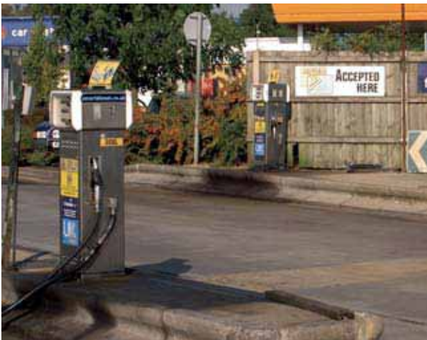
For real confidence that fuel is being measured and dispensed accurately, pumps should be calibrated once or ideally twice a year.
